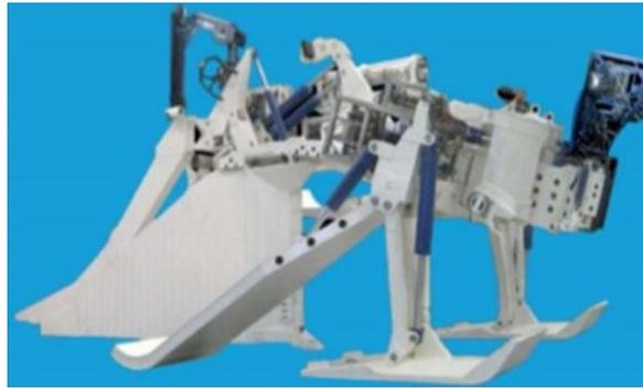
**Figure 5.11 Nexans CAPJET Jetter**
